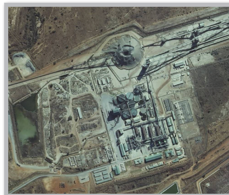
A zoomed in aerial image showing the mine processing plant with conveyor belt, buildings, mineral stock pile, dam and other infrastructure.
